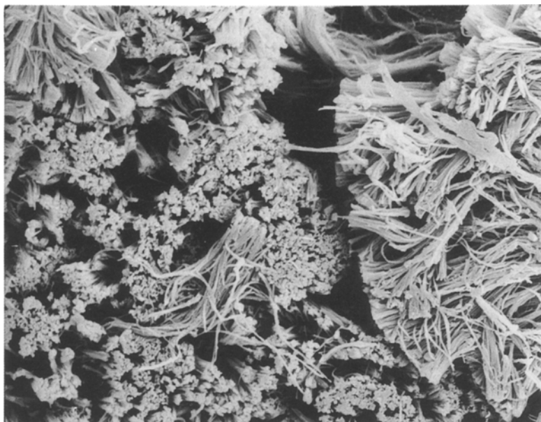
Figure 15 Polypyrrole grown from silver-painted Anotec membrane.
